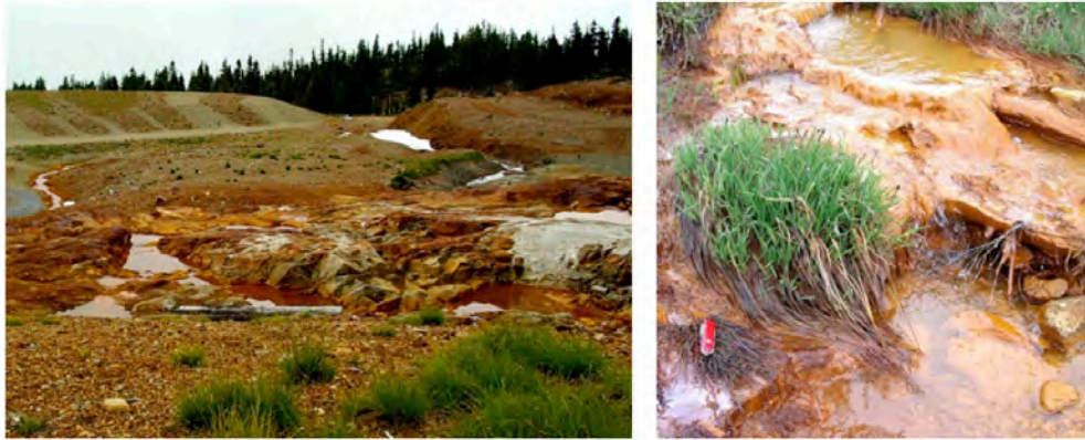
Figure 5.1.5: Exposed oxidizing and acid generating rocks and mine waste at the abandoned Mt. Washington Mine, B.C. (left), and an example of acid drainage downstream from the mine site (right).
